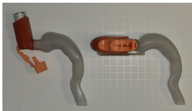
Fig. 2 Flovent HFA 134a MDI and Flovent Diskus DPI inserted into the characteristic MT geometry used for in vitro testing of aerosol deposition.
